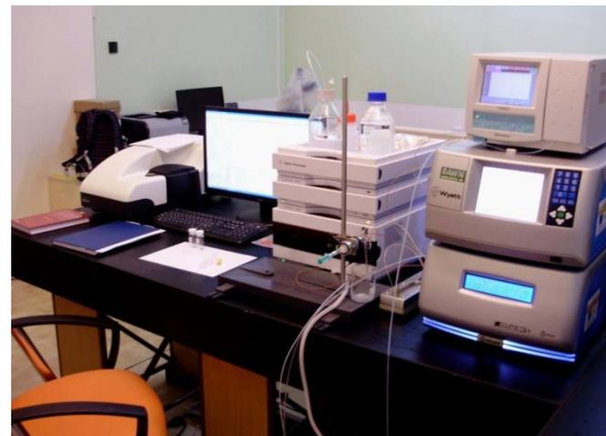
Fractionation of macromolecules or nanoparticles in asymmetric-flow field and subsequent simultaneous measurement of their concentration, size and molecular weight (Wyatt, USA). Extremely high resolution, for example, fig. to the left: BSA in form of a monomer, dimer, trimer, and higher associates.
